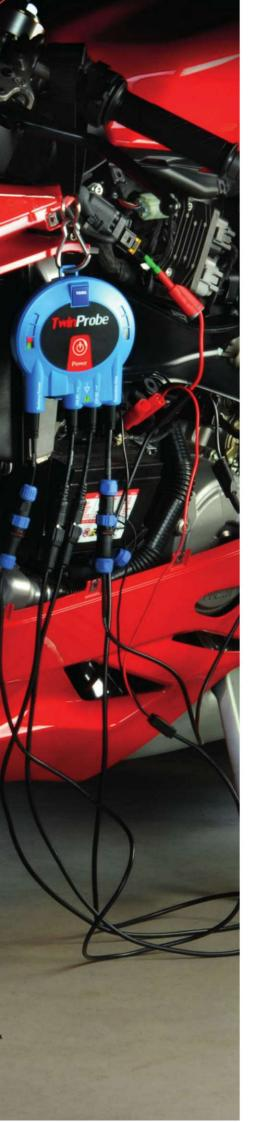
The UNIProbe and TwinProbe are two devices for acquiring the analogue and digital measurements needed for conventional diagnostic testing.
